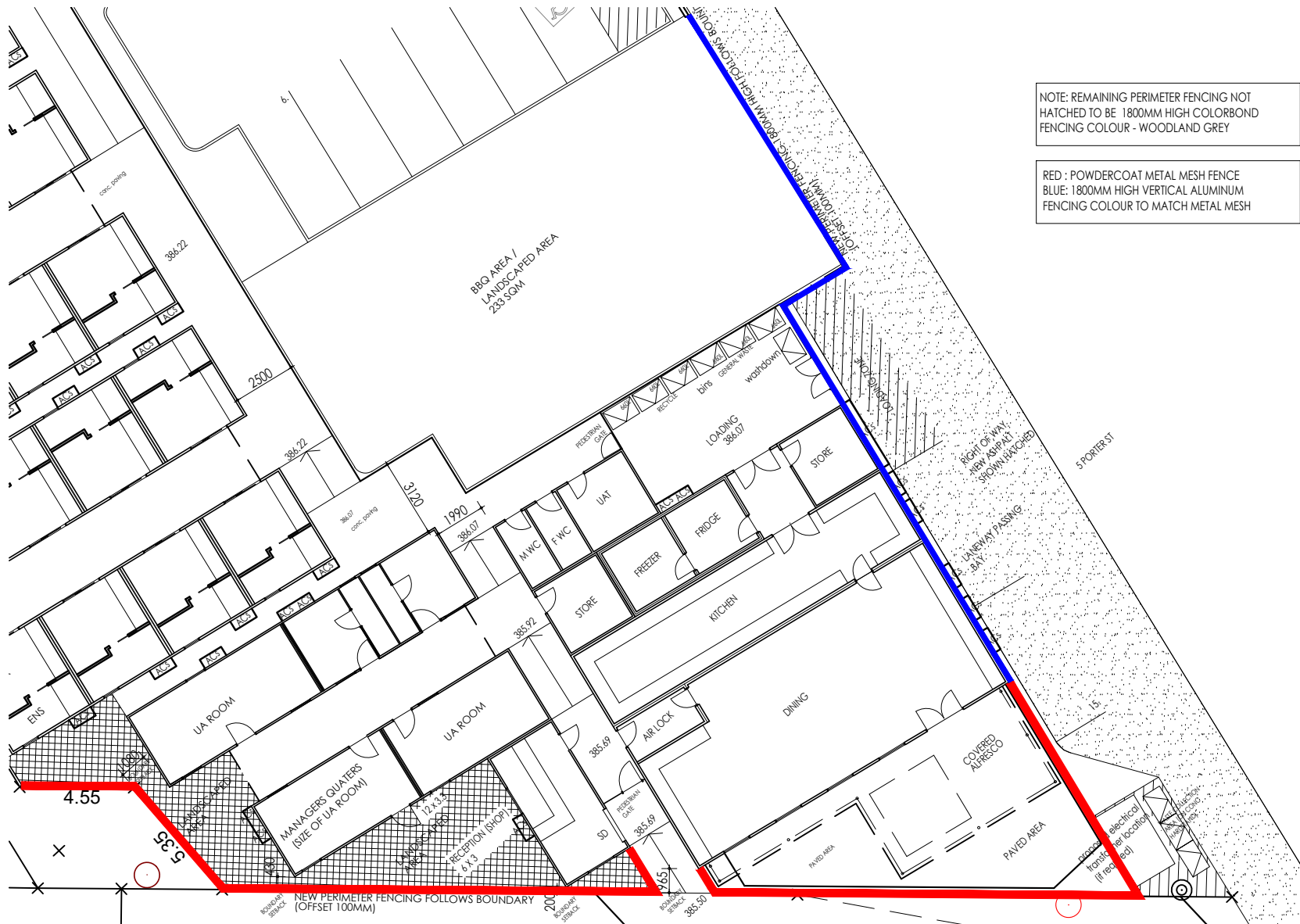
PLAN - FENCING EXTENT SCALE 1:200
